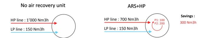
Depending on your machines, production and air network, switching OFF an HP compressor with ARS+ or a LP compressor with ARS can be considered, with significant savings on the compressor's maintenance
